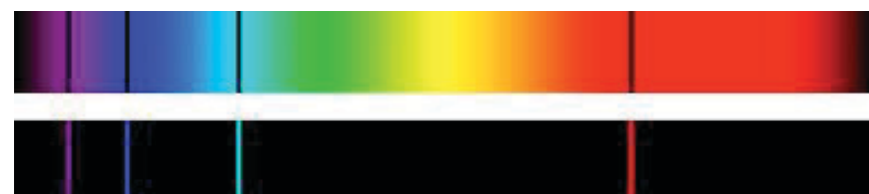
Absorption (above) and Emission spectra of hydrogen. The Emission lines are called the Balmer Series.
